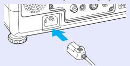
5 Connect the other end of the power cable to an earthed electrical outlet.
