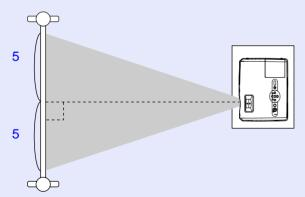
If it is not possible to set up the projector so that it is perpendicular to the screen, it can be set up at a slight vertical angle instead. You can adjust the upward projection angle of the projector to a maximum of 12° and the downward projection angle to a maximum of 4° by extending and retracting the front adjustable foot and rear adjustable feet.
