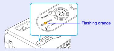
• The projected image gets darker or starts to deteriorate.
