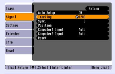
Tilt the [♠] button on the remote control or press the [♠] and [▷] buttons on the projector's control panel to adjust the tracking value until the vertical stripes disappear from the images.
