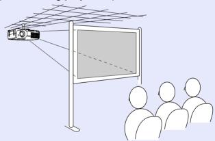
\* A special method of installation is required for suspending the projector from the ceiling. Please contact your supplier if you would like to use this installation method. The optional ceiling mount is required when installing the projector on the ceiling. • p.93
