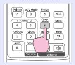
The current setting appears in the top-right corner of the screen each time the colour mode is changed.
