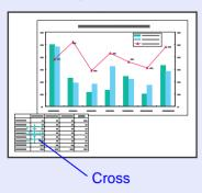
When the [⊕] button is pressed, the image is enlarged with the cross at its centre. When the [⊖] button is pressed, the enlarged image is then reduced.
