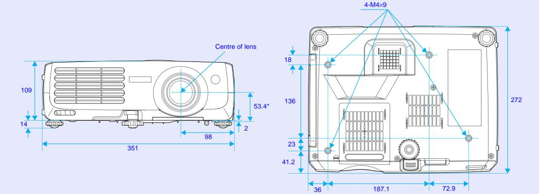
\*Distance from center of lens to suspension bracket fixing point
