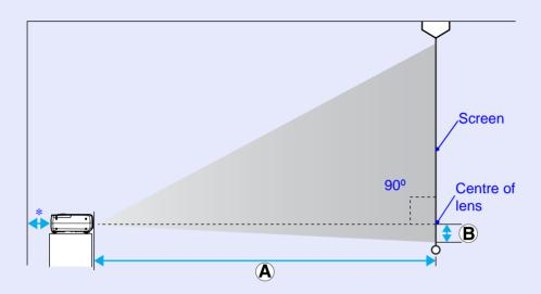
\* When installing against a wall, leave a space of about 20 cm (7.9 in.) between the projector and the wall.
