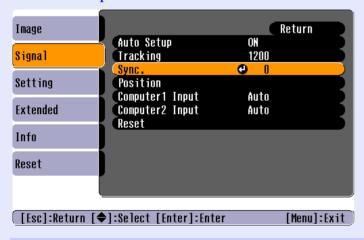
Tilt the [♠] button on the remote control or press the [♠] and [♠] buttons on the projector's control panel to adjust the synchronisation value until the flickering, fuzziness or interference disappears from the images.
